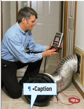
HVAC technicians or energy auditors can use diagnostic equipment to measure air leakage and air flow.
